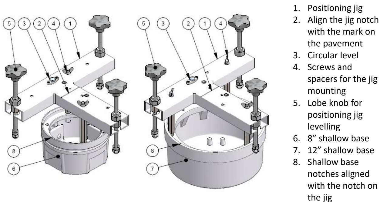
Figure 16 – Shallow base installation details
