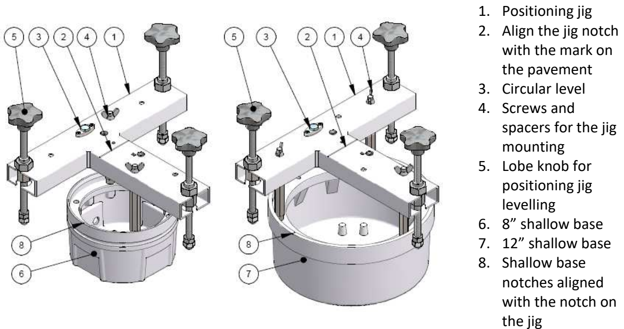
Figure 18 – Shallow base installation details
