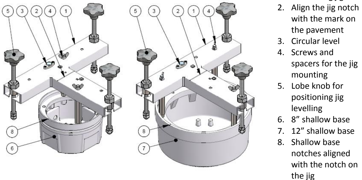
Figure 18 – Shallow base installation details
