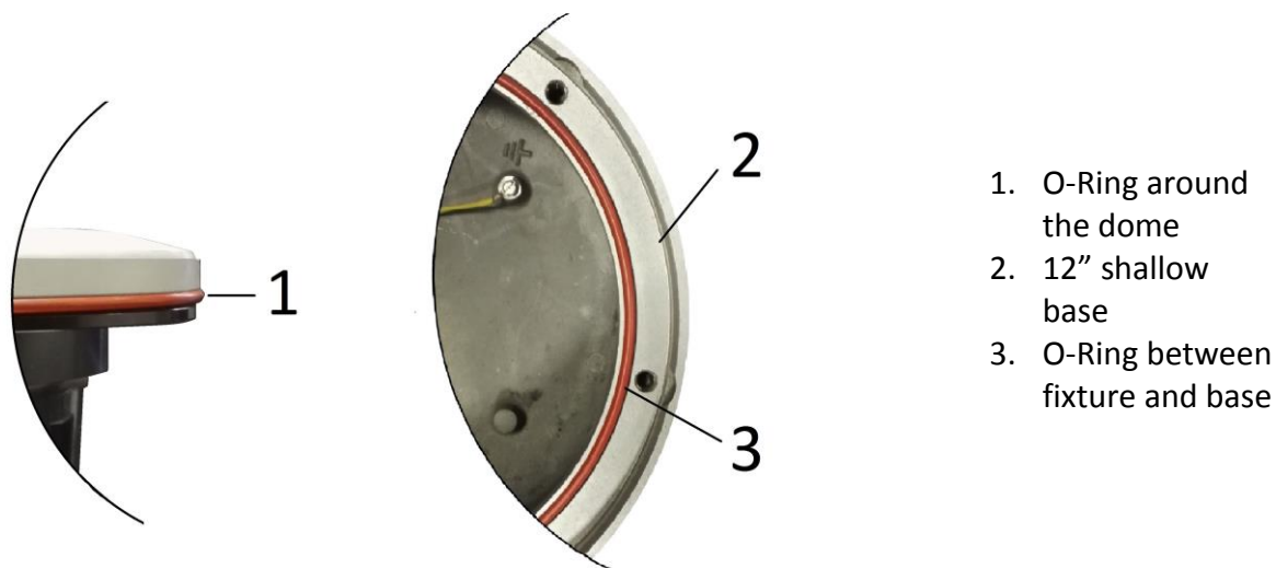
Figure 11 – Gaskets for 12" shallow base
